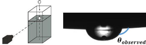
Figure 1: Contact angle analysis in a cuvette (left) and contact angle measurement of silanised bead (right)
