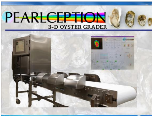
Figure 8. Automated 3D imaging system for oyster grading and sorting.
