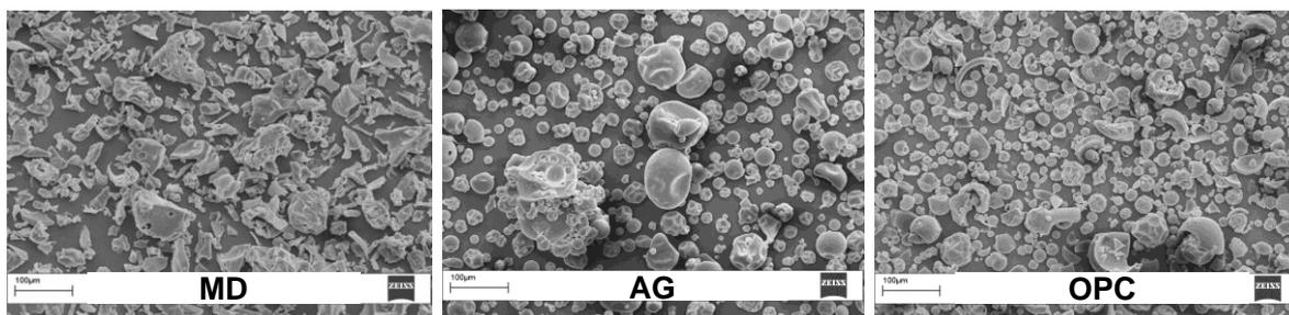
Figure 1: Scanning electron micrographs of samples of: Maltodextrin (MD); Arabic Gum (AG) and Proanthocyanidins (OPC).
