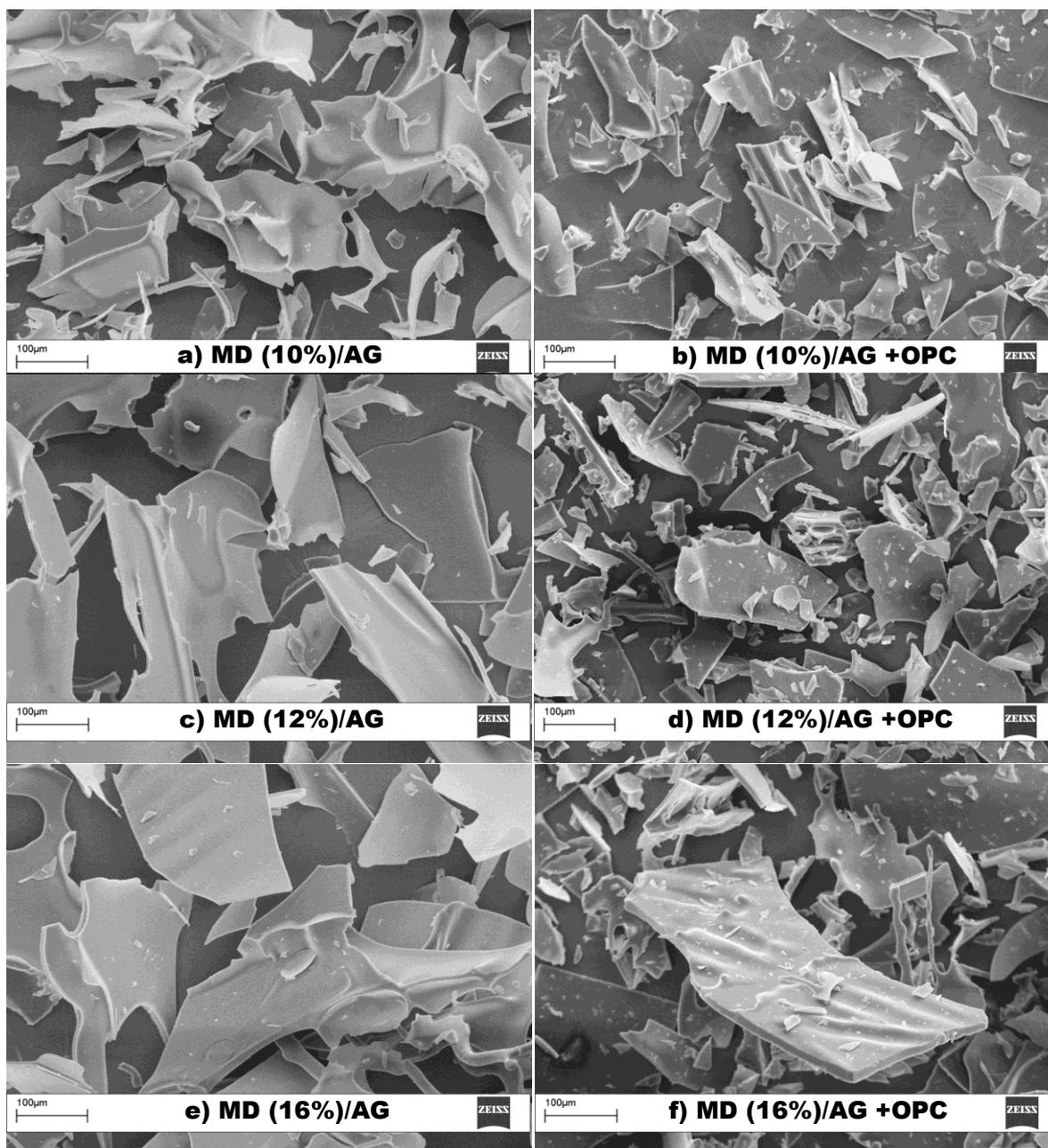
Figure 2: Scanning electron micrographs of samples of: a) MD/AG (10 / 4%); b) MD/ AG (10/ 4%) with OPC; c) MD/AG (12 / 4%); d) MD/ AG (12 / 4%) with OPC; e) MD/AG (16 / 4%); f) MD/AG (16 /4%) with OPC.
