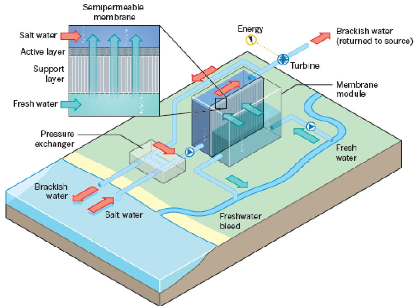
The plant ran from 2009 to 2012 at 10kW capacity with an initial membrane energy density of 1 W/m<sup>2</sup>
