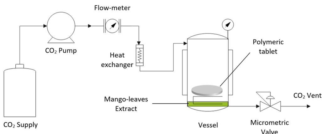
Figure 1: Schematic diagram of SSI pilot plant.
