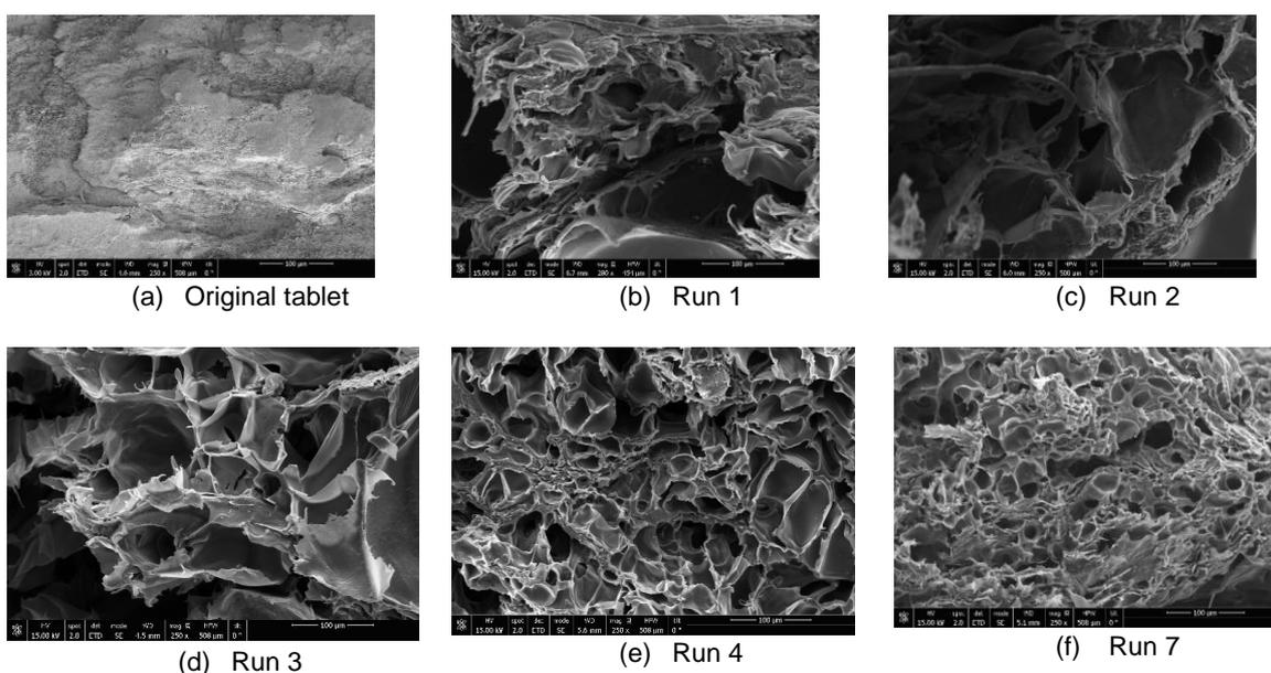
Figure 2: SEM images of (a) original PLGA/PEDOT:PSS tablet and formed scaffolds (1,2,3,4 and 7).
