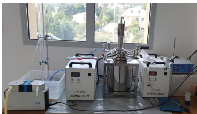
Figure 2: 500 ml HTC reaction system set up at University Kore of Enna.
