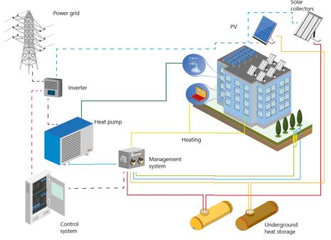
Figure 1: RESHeat system parts and topology
