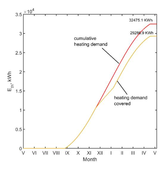
Figure 3: Cumulative energy flows for the test building – energy demands (upper curve) and RESHeat system supply (lower curve) for a 1 y cycle
