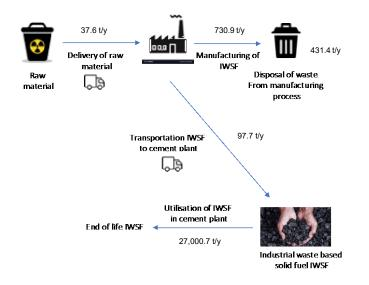
Figure 2: Baseline of carbon emission for hazardous waste based solid fuel: application in a cement kiln (Karpan et al., 2021)
