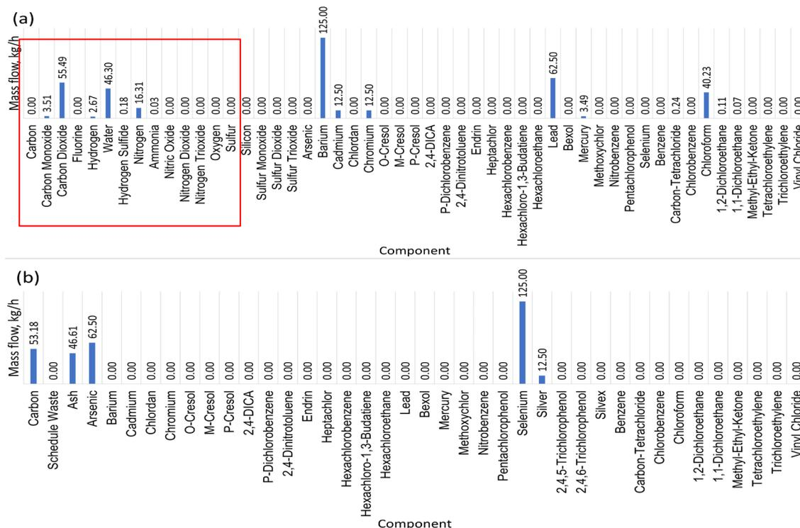
Figure 6: Outlet streams of the batch reactor at 500 °C (a) vapor stream (b) solid stream
