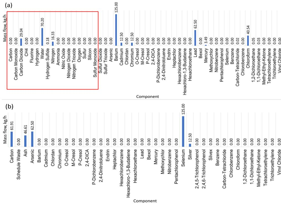
Figure 4: Outlet streams of the batch reactor at 100 °C (a) vapor stream (b) solid stream
