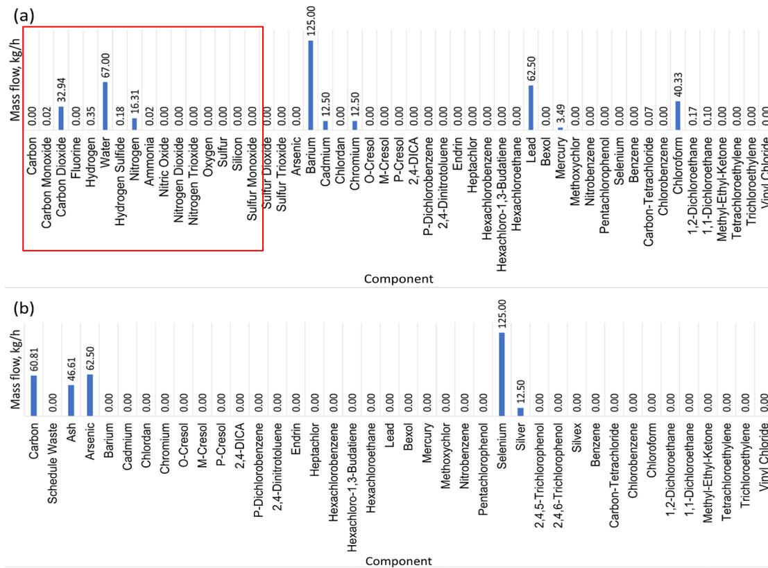
Figure 5: Outlet streams of the batch reactor at 300 °C (a) vapor stream (b) solid stream
