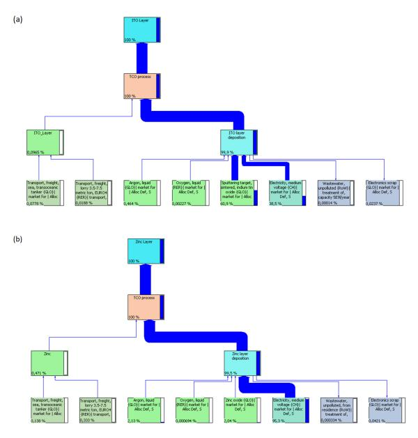
Figure 1: Process tree for a) ITO and b) ZnO coating deposited by PVD technique.
