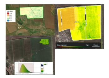
Figure 4: Calculation of NDVI index. Alfalfa crop: 1 - based on Landsat 8 satellite imagery, 2 - one soil web application, 3 - based on DJI Phantom 4 Multispectral aerial imagery
