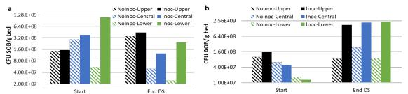
Figure 4. Bacterial abundance in upper, central and lower sections of uninoculated (Nolnoc) and inoculated (Inoc) biofilters. (a) sulphur-oxidizing bacteria (SOB); (b)ammonia-oxidizing bacteria (AOB).
