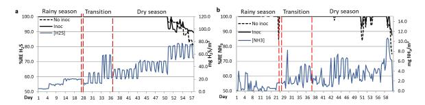
Figure 2. Biofiltration of (a)  $H_2S$  and (b)  $NH_3$  under transitory conditions of gas concentration. Black lines represent the removal efficiency (%ER) of inoculated (Inoc) and not inoculated biofilters (No inoc). The continuous blue line indicates the inlet gas concentration. Dotted red vertical lines indicate the change in the type of transient condition applied. From day 25 to day 30 there was a stabilisation period at low gas concentration after a biofilter bed washing.
