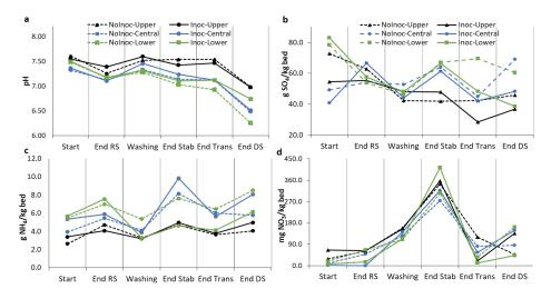
Figure 3. Monitoring of  $H_2S$  and  $NH_3$  elimination products in upper, central and lower sections of uninoculated (Nolnoc) and inoculated (Inoc) biofilters. (a) pH variation; (b) concentration of produced sulphate; (c) accumulated ammonium concentration; (d) concentration of produced nitrate. RS, Rainy season; Washing: sample was taken after bed washing; Stab, stabilisation stage; Trans, transition stage; and DS, dry season.
