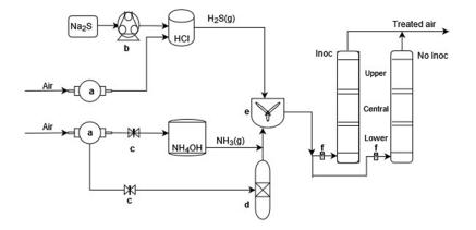
*Figure 1. Gas generation system and laboratory-scale biofilters. a. Vacuum pump; b. Peristaltic pump; c. Valves; d. Humidifier; e. Mixing chamber; f. Flowmeters; Inoc. inoculated biofilter; No inoc, Uninoculated biofilter.*
