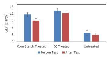
Figure 5. GLP Before and After Biodegradability Test
