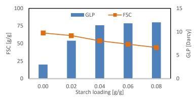
Figure 2. Free Swell Capacity and GLP of Untreated and Corn Starch treated SAP
