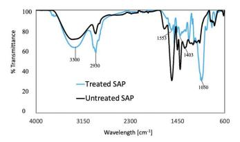
Figure 1. FTIR Results for untreated SAP and corn starch treated SAP
