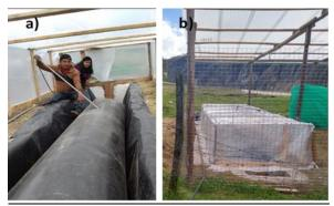
Figure 2: a) Tubular biodigester and b) Greenhouse
