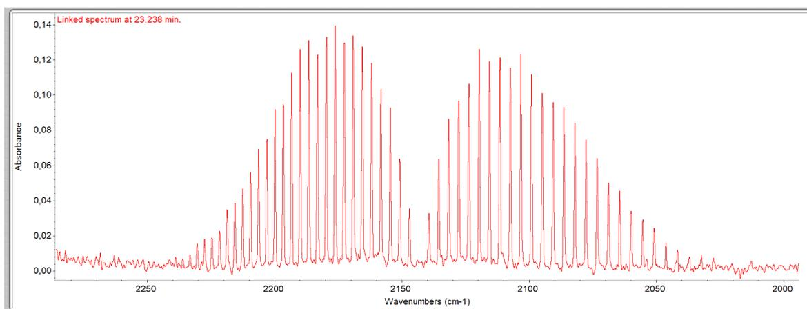
Figure 2: PLA filament spectrum of carbon monoxide, 22nd minute
