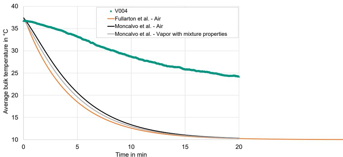
Figure 3: Temporal progression of the average tank temperature of experiment V004 (triangled line) and the literature models of Fullarton et al. (Fullarton et al. 1987; Fullarton 1986) (orange solid line) and Moncalvo et al. (Moncalvo et al. 2016) for dry air (black solid line) and moist air with mixture properties (grey solid line)
