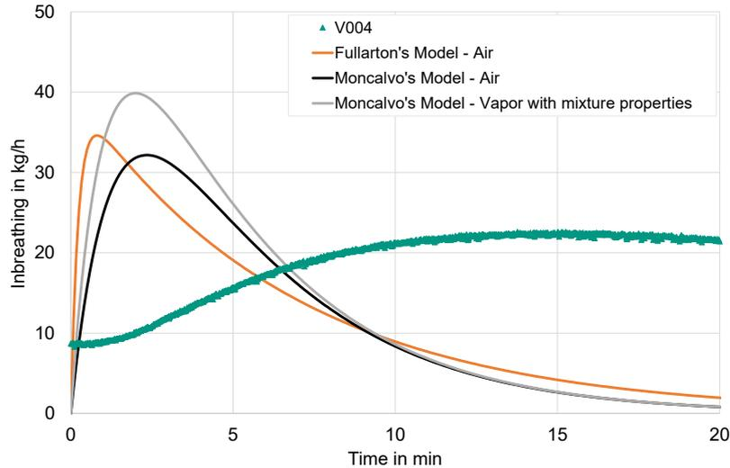
Figure 2: Inbreathing rate over time of experiment V004 (triangled line) and the literature models of Fullarton et al. (Fullarton et al. 1987; Fullarton 1986) (orange solid line), Moncalvo et al. (Moncalvo et al. 2016) for dry air (black solid line) and moist air with mixture properties (grey solid line)
