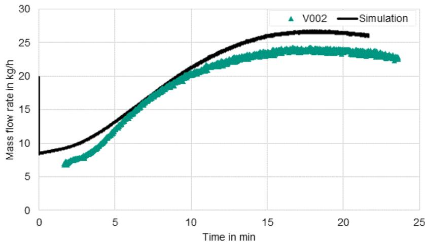
Figure 4: Tank breathing mass flow rate from CFD simulation (black solid line) and experiments (green triangled line).
