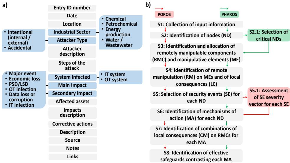
Figure 1: a) Structure of the developed database (grey boxes: free text fields; light blue boxes: itemized fields); b) Flowchart of POROS (red arrows) and PHAROS (green arrows)
