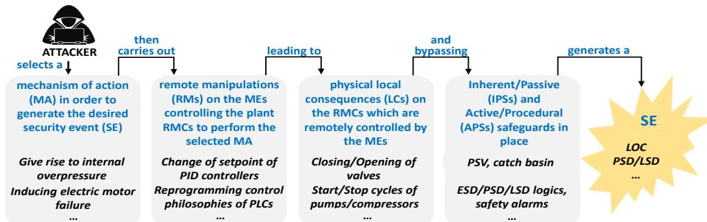
Figure 2: Core mechanism of PHAROS and POROS methodologies
