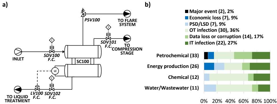
*Figure 3: a) Process Flow Diagram (PFD) of the SUC; b) (results from PIA) Share of the impacts of the CSIs recorded vs the industrial sectors*
