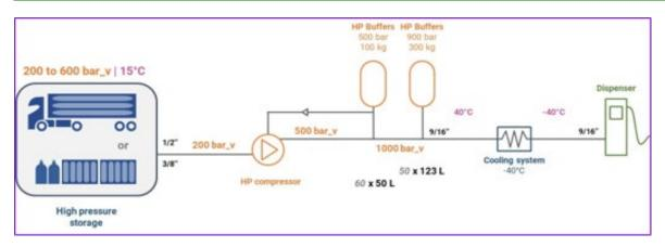
Figure 1: Example of the studied configuration (configuration 1)
