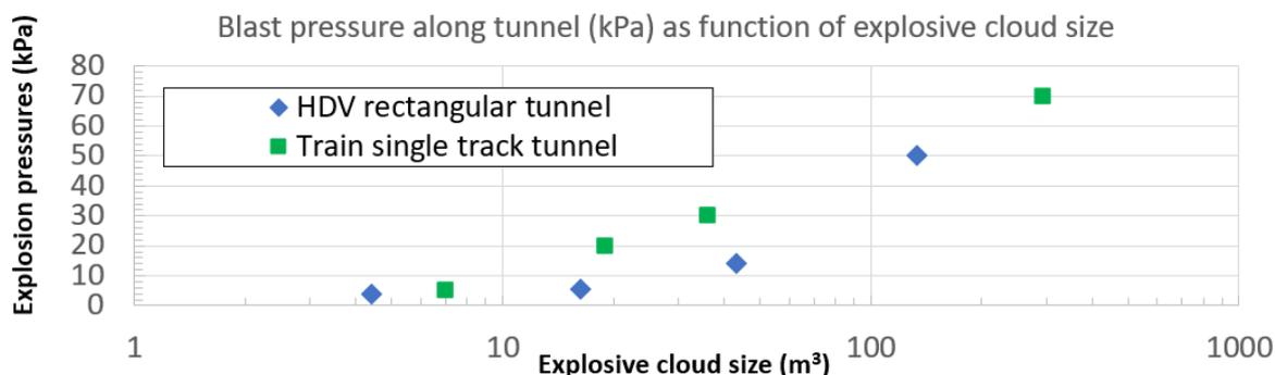
Figure 7: Explosion pressure along tunnels as function of explosive cloud sizes.
