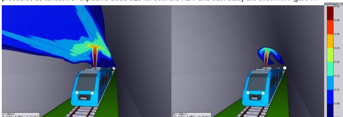
Figure 5: Flammable cloud from 4.5 mm TPRD release with initial rate 286 g/s for train at rest (left) and at 36 km/h (right).
