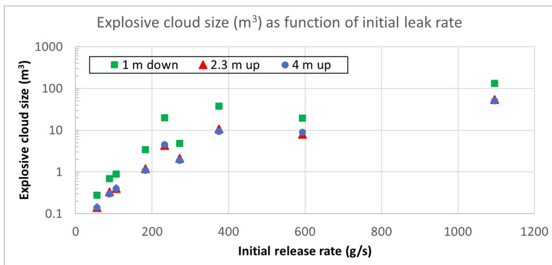
Figure 3: Maximum predicted equivalent stoichiometric cloud size  $Q_9$  (m<sup>3</sup>) plotted as function of initial leak rate for all simulations performed in the rectangular tunnel.
