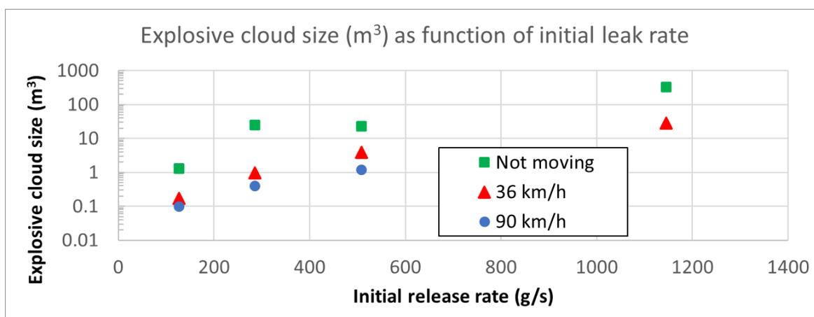
Figure 6: Maximum predicted equivalent stoichiometric cloud size  $Q_9$  (m<sup>3</sup>) plotted as function of initial leak rate for all simulations performed in the single-track railway tunnel.
