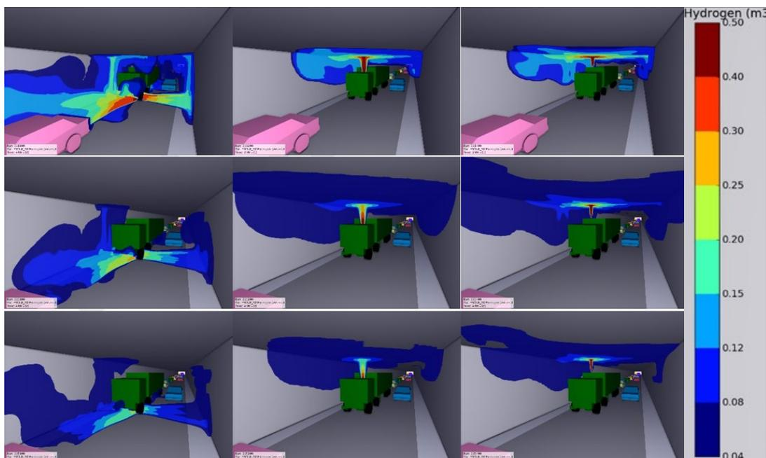
Figure 2: Illustration of hydrogen concentration at maximum reactivity for releases from a 10 kg tank with 1-minute releases in a rectangular tunnel (upper – 593 g/s), 3-minute releases in a rectangular tunnel (middle – 182 g/s) and 5-minute releases in a rectangular tunnel (lower – 106 g/s) for releases downwards from 1 m elevation (left), upwards from 2.3 m elevation (centre) and upwards from 4 m elevation (right).
