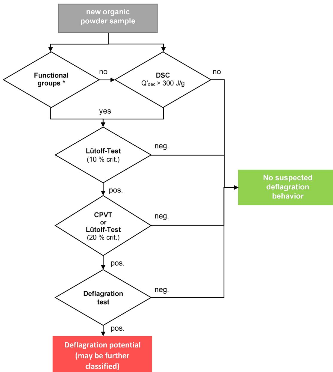
Figure 4: Suggested screening procedure to identify deflagration potential of bulk solids (\* Functional groups according to Appendix 6 of the UN DG Manual of Test and Criteria)
