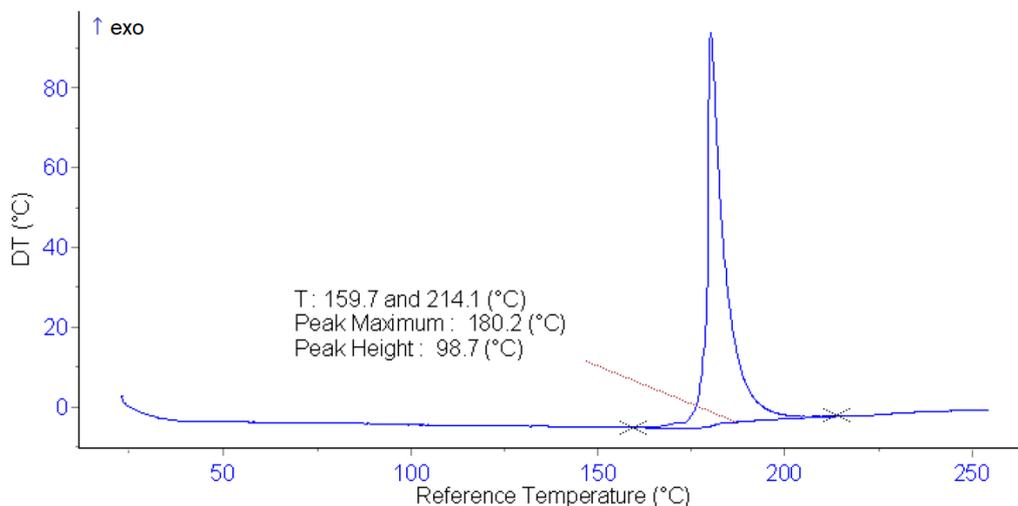
Figure 3: Thermogram of a Lütolf-Test with a sample in which the temperature difference  $DT$  is plotted against the reference temperature
