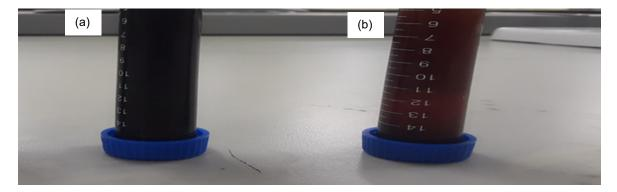
Figure 2: Illustration colour differences between (a) SCG oil extracted using 2-MeTHF (b) SCG oil extracted using hexane.
