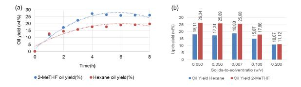
Figure 1: Illustration the effects (a) of extraction time and (b) solvent to solids ratio on the oil yield
