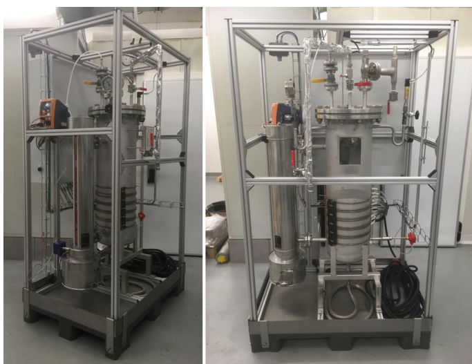
Figure 6: Experimental Ammonia generator (under construction).
