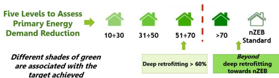
Figure 2: Five levels to assess primary energy demand reduction; the last step (nZEB Standard) stands for “nearly Zero-Energy Building”, that is a building with a primary energy consumption near zero
