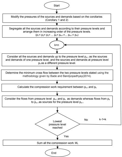
Figure 2: Targeting algorithm for minimizing compression work in a multi-pressure level heat supply network
