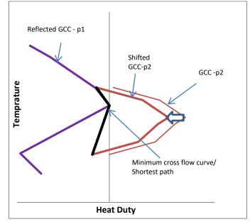
Figure 3: Determination of minimum cross-flow between two GCCs
