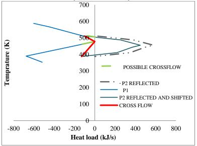
Figure 2: Determination of cross-flow for an illustrative example
