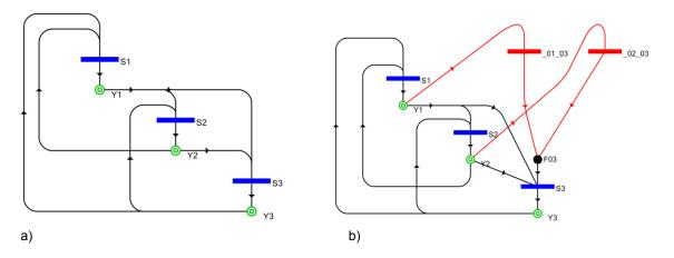
Figure 1: P-graph representation of an economic system with (a) fixed I-O ratios and (b) flexible I-O ratios for partial substitution
