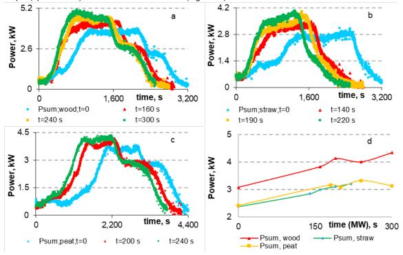
Figure 2: The effect of MW pre-treatment time of wood, straw, and peat pellets on kinetics of the heat output (a-c) and average values of the heat output from the setup in the flame reaction zone (d).
