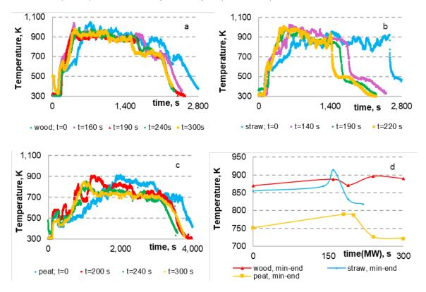
Figure 1: The effect of MW irradiation time of wood (a), straw (b) and peat (c) pellets on dynamics and average values of the flame temperature (d).
