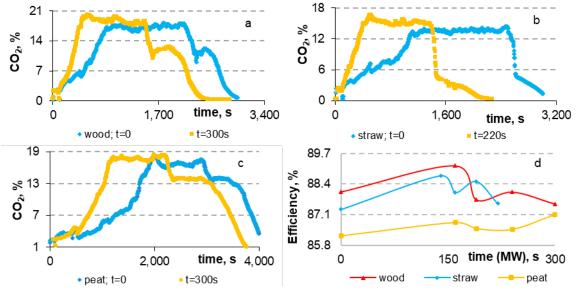
Figure 3: The effect of MW pretreatment time on the formation of  $CO_2$  emission for wood (a), straw (b) and peat (c) pellets and the average value of combustion efficiency (d).
