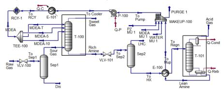
Figure 4: Process flow diagram for Sahel sweetening unit by Aspen HYSYS software.
