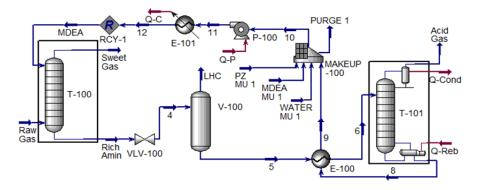
Figure 3: Process flow diagram for Alestiklal sweetening unit by Aspen HYSYS software.
