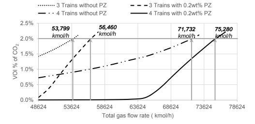
Figure 2: Raw gas flow rate vs. CO<sub>2</sub> concentration (vol %) in the sweet gas stream for different scenarios
