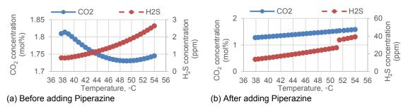
Figure 5: Effect of lean solvent temperature on sweet gas composition.
