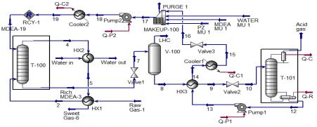
Figure 1: Process flow diagram for Mellitah sweetening unit by Aspen HYSYS software
