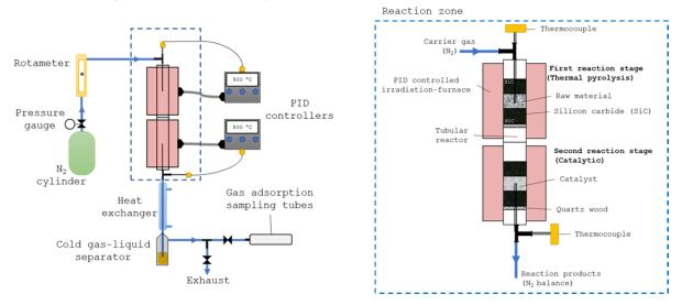
Figure 1: Scheme of the experimental test bench for thermal and thermo-catalytic pyrolysis.
