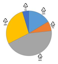
Figure 2: Composition of the mixed municipal plastic sample (SDU sample) used in this work.
