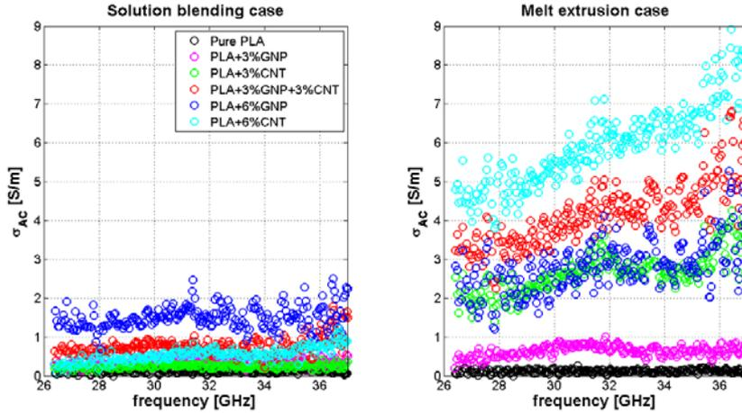
Figure 4: AC electrical conductivity for SB (left) and ME (right) filament samples compared with pure PLA
