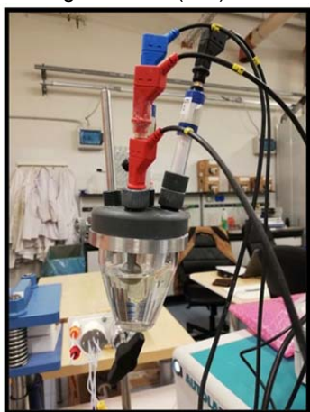
Figure 2: Electrochemical cells used for corrosion tests.
