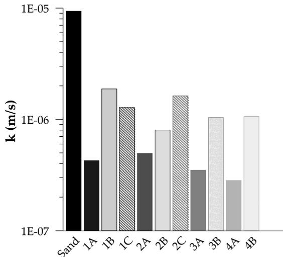
Figure 2: Hydraulic conductivity values for each mix and untreated sand
