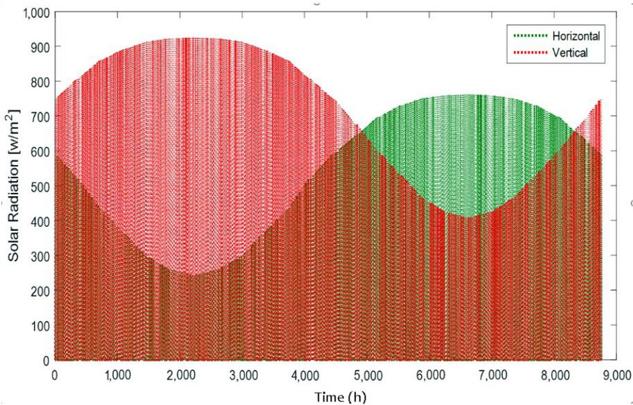
Figure 2: The horizontal and vertical solar irradiance during a year
