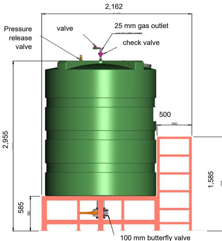
Figure 5: The design of the pilot-scale AD for Eco-park UTM
