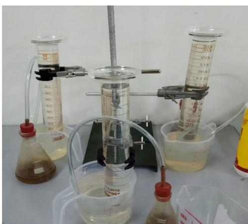
Figure 1: Experimental setup for lab-scale AD
