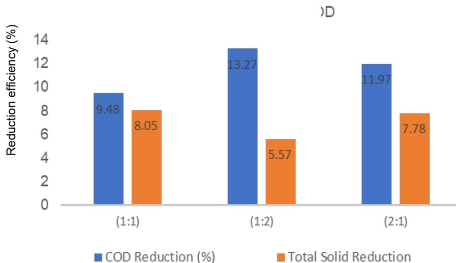
Figure 4: COD and TS reduction efficiency for three samples with different ratios of FVW and POME
