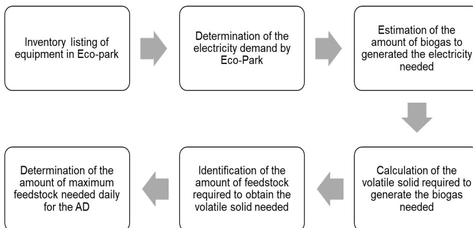
Figure 2: Process flow in designing the pilot-scale AD for Eco-park UTM
