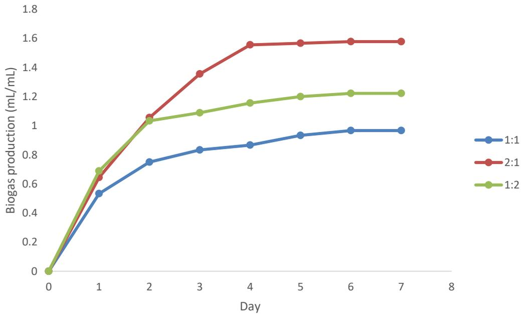
Figure 3: Daily biogas production (mL of biogas/mL of feed) for three samples with different ratios of FVW and POME
