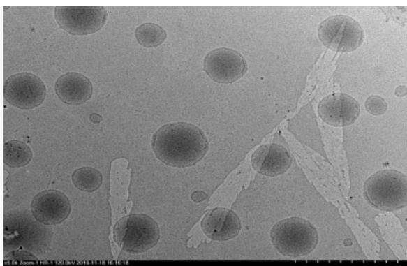
*Figure 2: Morphology of NLC-lemongrass oil formulation A4 observed under the transmission electron microscopy (Magnification of 5,000).*
