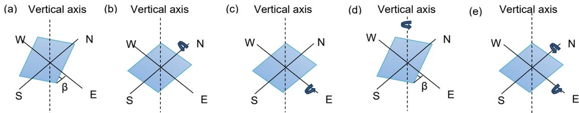
Figure 1: PV system with (a) fixed tilt (b) EWSAT (c) NSSAT (d) VSAT (e) DAT
