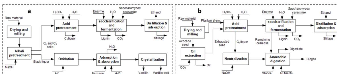
Figure 1: Process block diagram of (a) Sc.1, (b) Sc.4 and 5.
