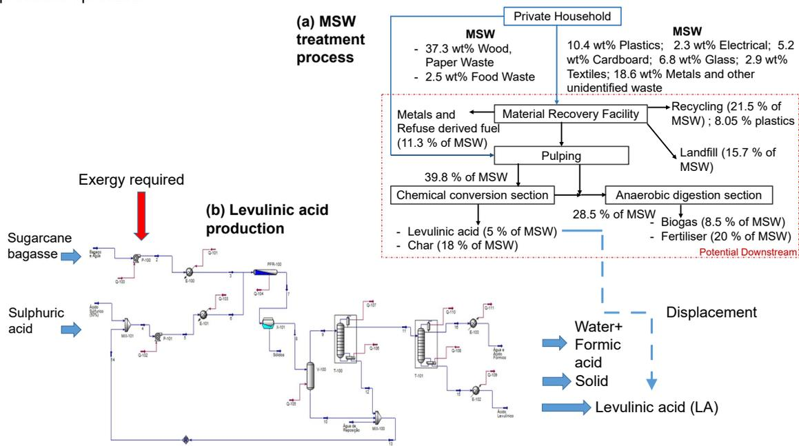
Figure 2: Input-output mass balances for MBCT of MSW, adapted from (Sadhukhan et al., 2016). LA production process is adapted from (Gaudereto et al., 2017)
