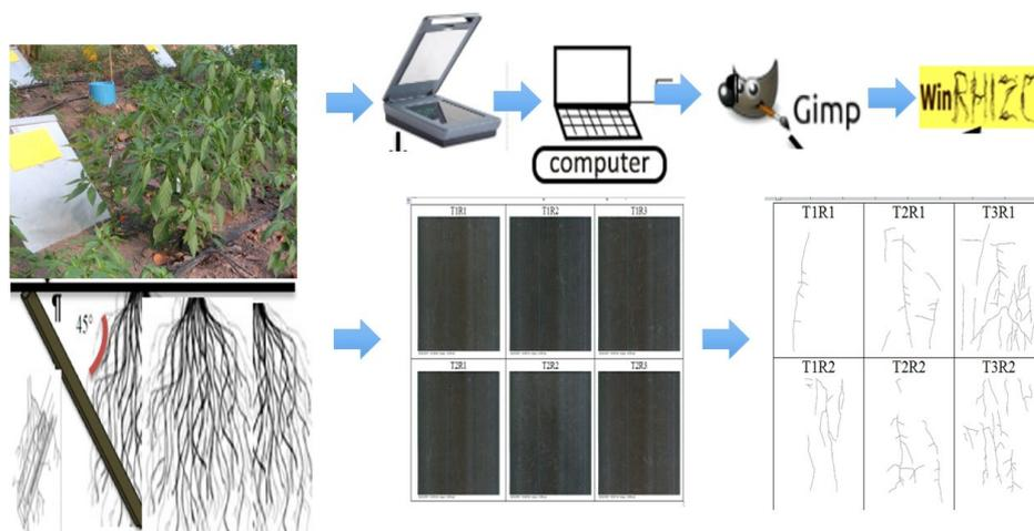
Figure 2: Schematic diagram of fine root measurement using minirhizotron techniques.
