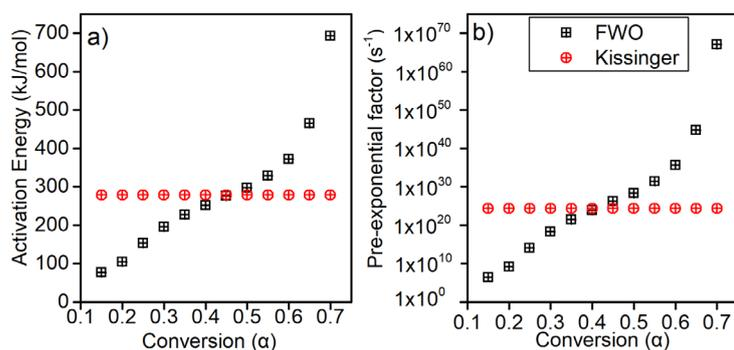
Figure 3: (a) Activation energy and (b) pre-exponential factor obtained using FWO and Kissinger methods in relation to the conversional level
