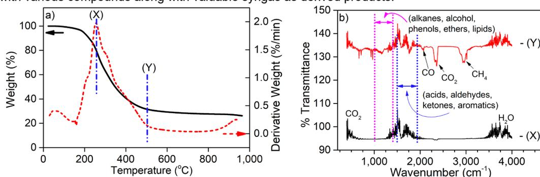
Figure 1: Thermal degradation of sludge cake at 20 °Cmin<sup>-1</sup> in (a) mass loss and derivative mass loss curve along with (b) volatile evolved as detected by FTIR
