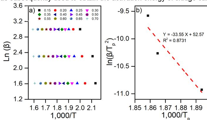
Figure 2: Linear plot for (a) FWO and (b) Kissinger methods
