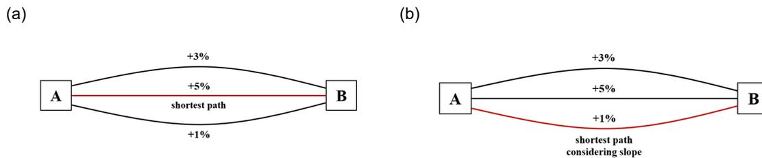
Figure 1: (a) existing route algorithm, (b) route algorithm considering slope
