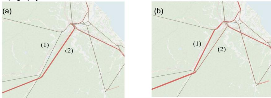
Figure 2: (a) existing route algorithm, (b) route algorithm considering slope
