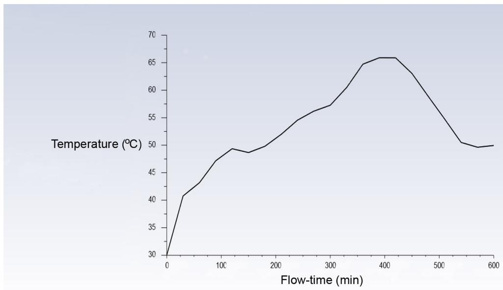
Figure 2: Simulation temperature profile inside the SGHD from 7:00 AM to 6:00 PM
