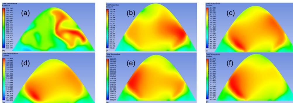
Figure 5: Temperature distribution of moist air in the volume of the SGHD at various times: (a): 8:00 AM; (b): 10:00 AM; (c): 12:00 PM; (d): 1:00 PM; (e): 2:00 PM; and (f): 4:00 PM
