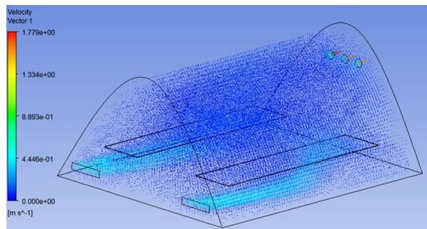
Figure 6: Velocity vectors of the airflow inside the SGHD
