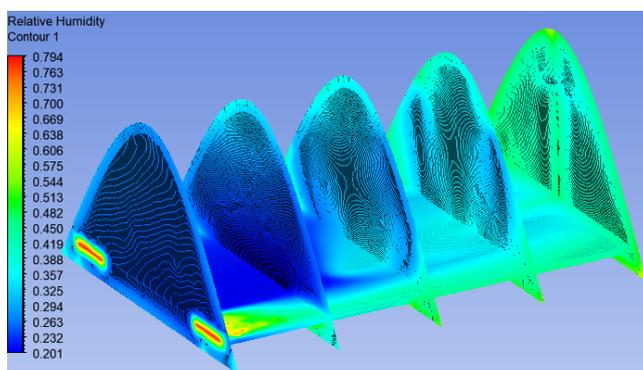
Figure 8: RH distribution of moist air in the volume of the SGHD at various location
