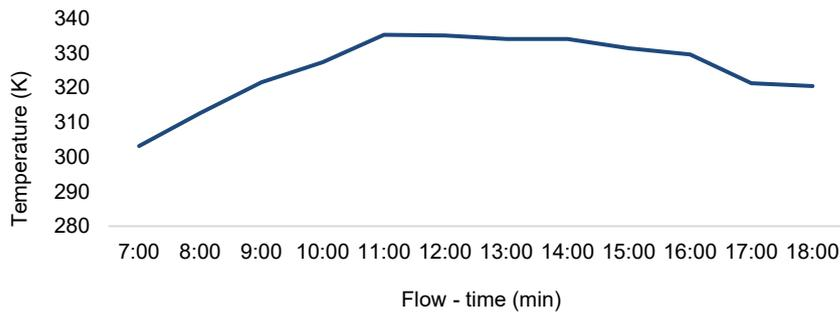
Figure 3: Experimental temperature inside the SGHD from 7:00 AM to 6:00 PM
