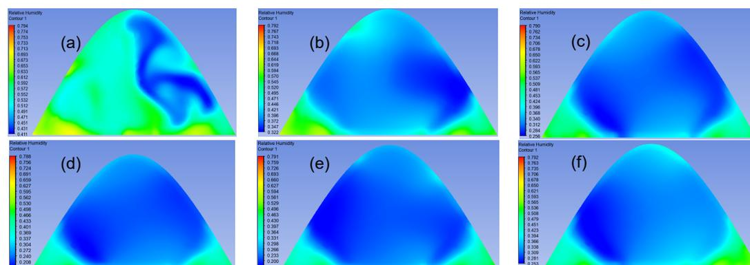
Figure 7: RH distribution of moist air in the volume of the SGHD at various time: (a): 8:00 AM; (b): 10:00 AM; (c): 12:00 PM; (d): 1:00 PM; (e): 2:00 PM; and (f): 4:00 PM
