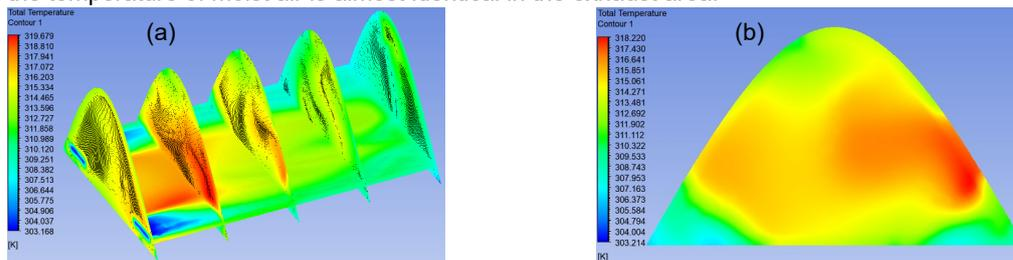
Figure 4: Temperature distribution of moist air in the volume (a) at various location and (b) in the middle of the SGHD
