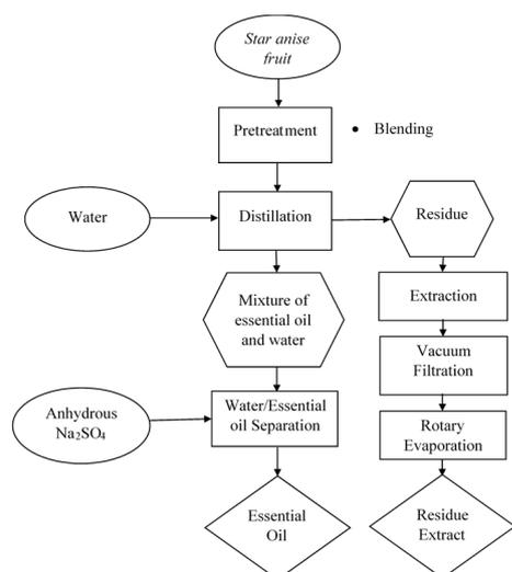
Figure 1: Star anise essential oil distillation and residue extraction procedure.
