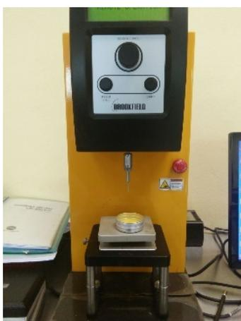
Figure 3: The hardness of lip balm was analysed using Ametek Brookfield CT-3 Texture Analyzer
