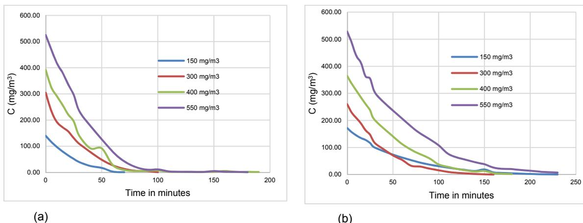
Figure 3: Kinetics of cyclohexane degradation in a batch reactor with (a) TiO<sub>2</sub> on cellulosic support and (b) TiO<sub>2</sub> on optical fibers
