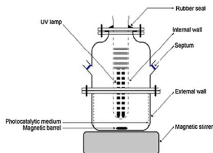
Figure 1: Diagram of a discontinuous photocatalytic reactor
