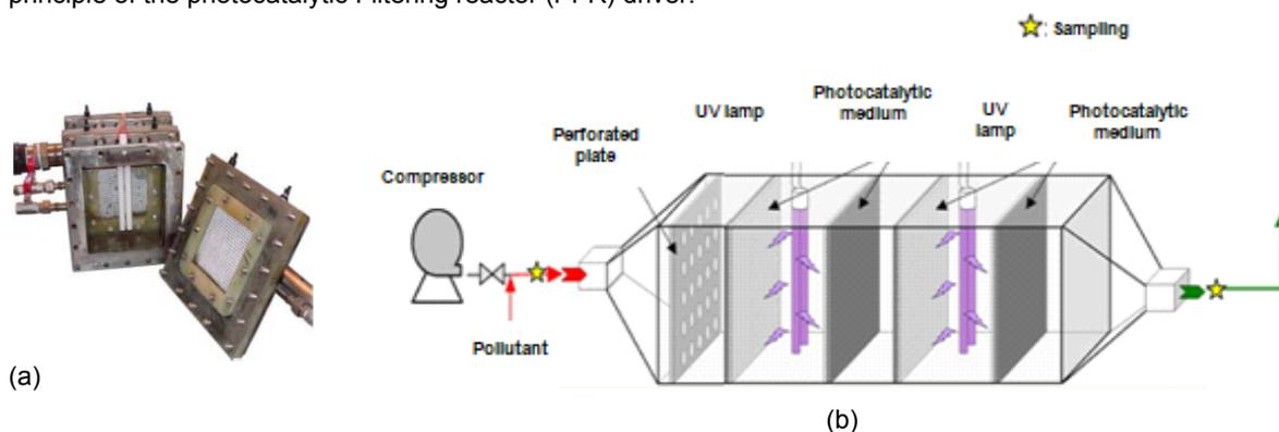
Figure 2.: a) photocatalytic Filtering reactor (PFR) and b) Schematic diagram
