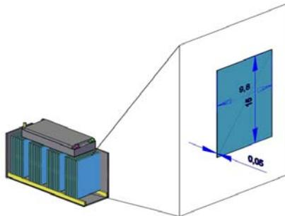
Figure 2. Fixing the electrodes inside the oxyhydrogen gas generating device
