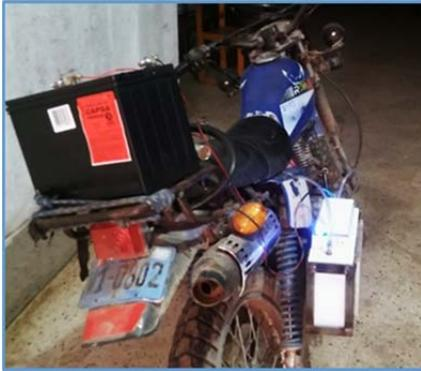
Figure 8. Adaptation of the oxyhydrogen gas generating system on board the vehicle
