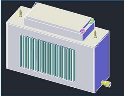
Figure 1. Oxyhydrogen gas generating device
