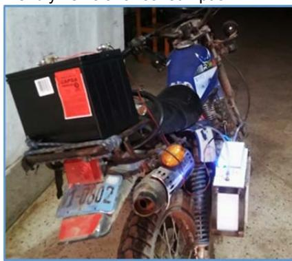
Figure 8. Adaptation of the oxyhydrogen gas generating system on board the vehicle
