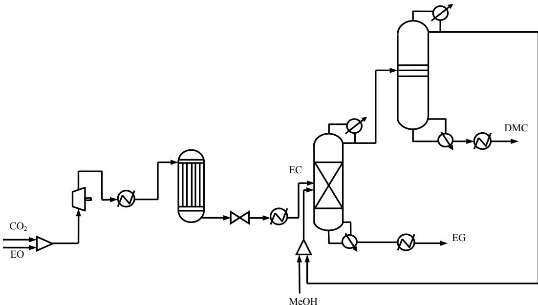
Figure 1. The simplified flowsheet of DMC production from CO<sub>2</sub> catalysed by ionic liquid (ILS process).
