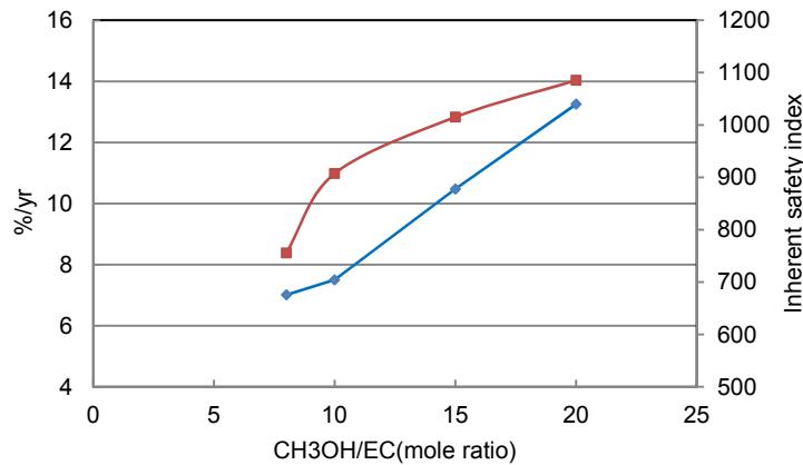
Figure 4. The effect of the mole ratio of methanol to EC on ROI and inherent safety index.
