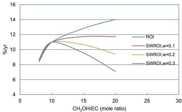
Figure 5. The effect of the ratio of methanol to EC on SWROI at different weighting factor of safety.
