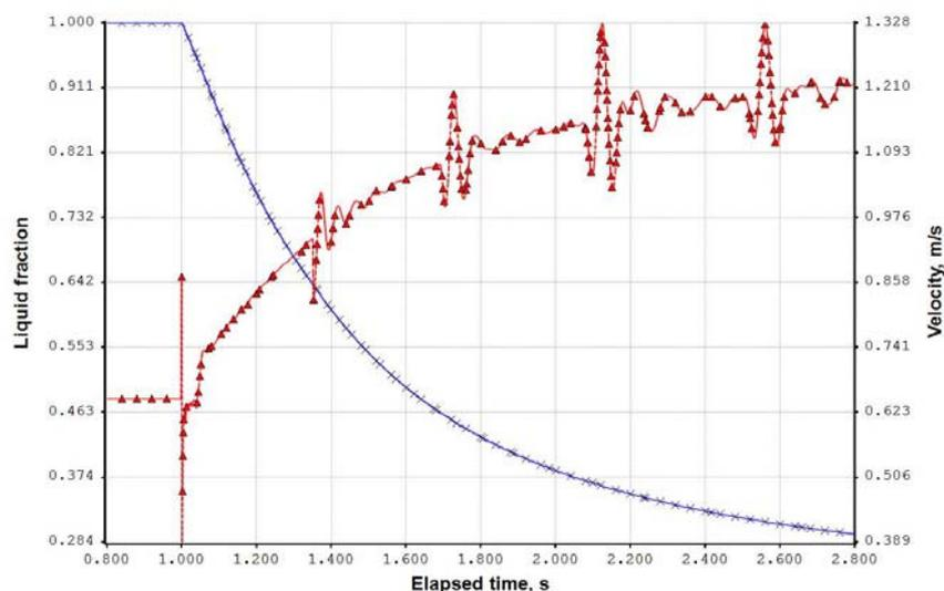
Figure 6: Liquid volume fraction (x) and fluid velocity (Δ) at 1 m after tube rupture
