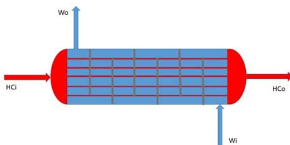
Figure 1: Shell & Tube heat exchanger schema: hot gas (red) and cooling water (blue)
