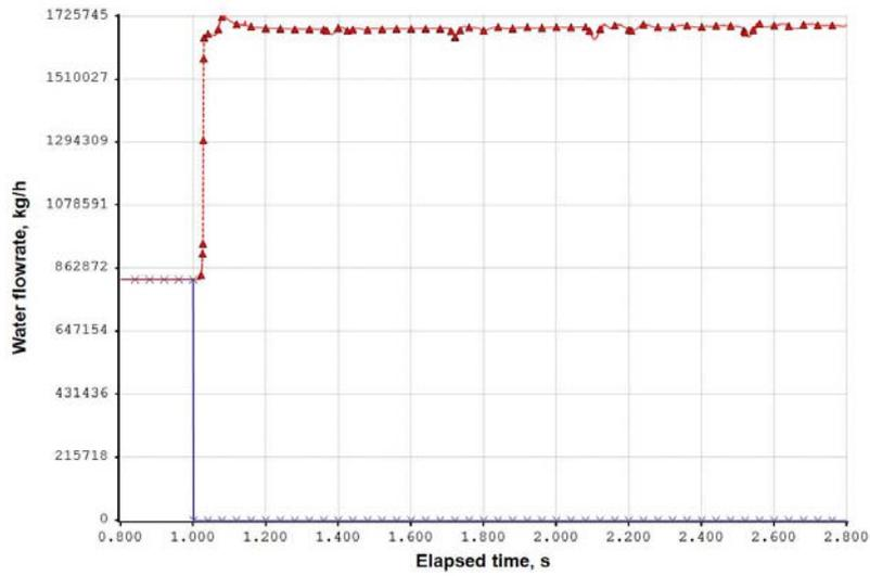
Figure 4: Inlet (x) and outlet (Δ) cooling water flow flowrate
