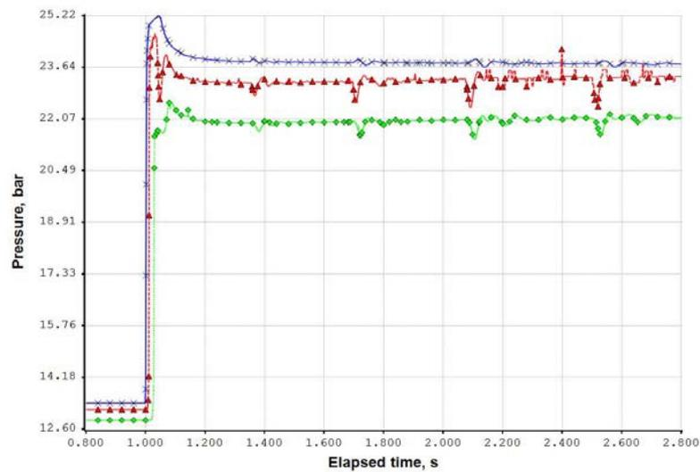
Figure 5: Calculated pressures in the shell at water flow points, inlet (x), middle (Δ) and outlet (◇) points
