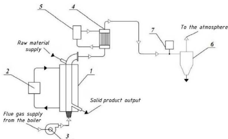
Figure 1: Scheme of experimental set-up for studying the oxidative torrefaction process of sunflower husks. 1-fluidized bed reactor, 2-electric boiler, 3-smoke exhauster, 4-heat exchanger, 5-storage tank, 6-mechanical cleaning in cyclone, 7-gas analyzer
