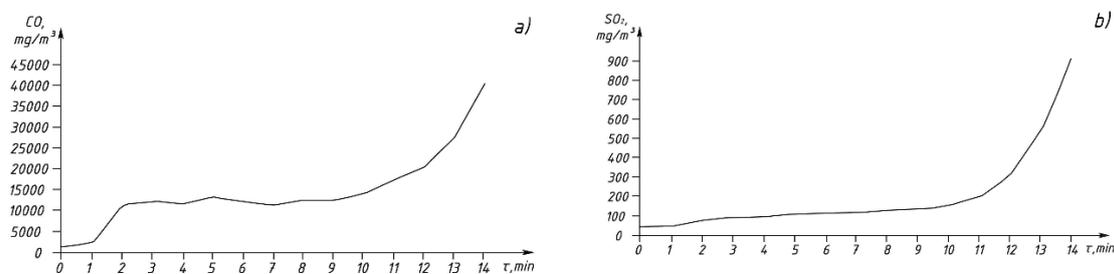
Figure 4: a) Change in carbon monoxide concentration in non-condensable gaseous products during sunflower husk torrefaction in fluidized bed, b) Change of sulfur dioxide concentration in non-condensable gaseous products during sunflower husks torrefaction process in fluidized bed
