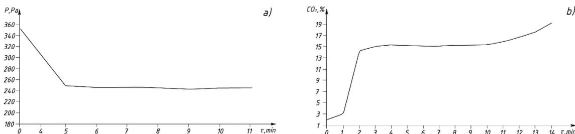
Figure 3: a) Change in pressure drop in fluidized bed + gas distribution system during torrefaction of sunflower husks, b) Change in carbon dioxide concentration in non-condensable gaseous products at torrefaction process of sunflower husks in a fluidized bed
