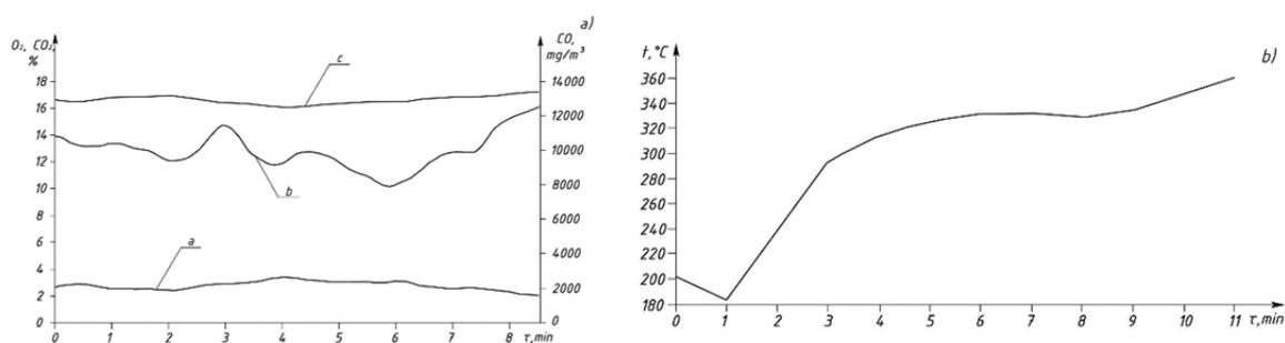
Figure 2: a) Content of flue gases at the entrance to fluidized bed of sunflower husks (a - oxygen content, b - carbon monoxide content, c - carbon dioxide content), b) Change in temperature of husk fluidized bed in torrefaction process
