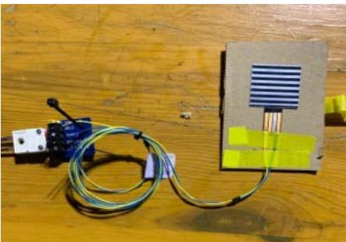
Figure 3: The Captec Radiant Flux sensor.
