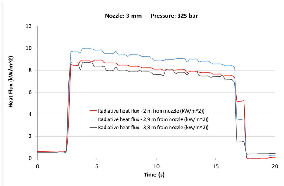
Figure 6: Heat Flux for 3 mm orifice at 325 bar.
