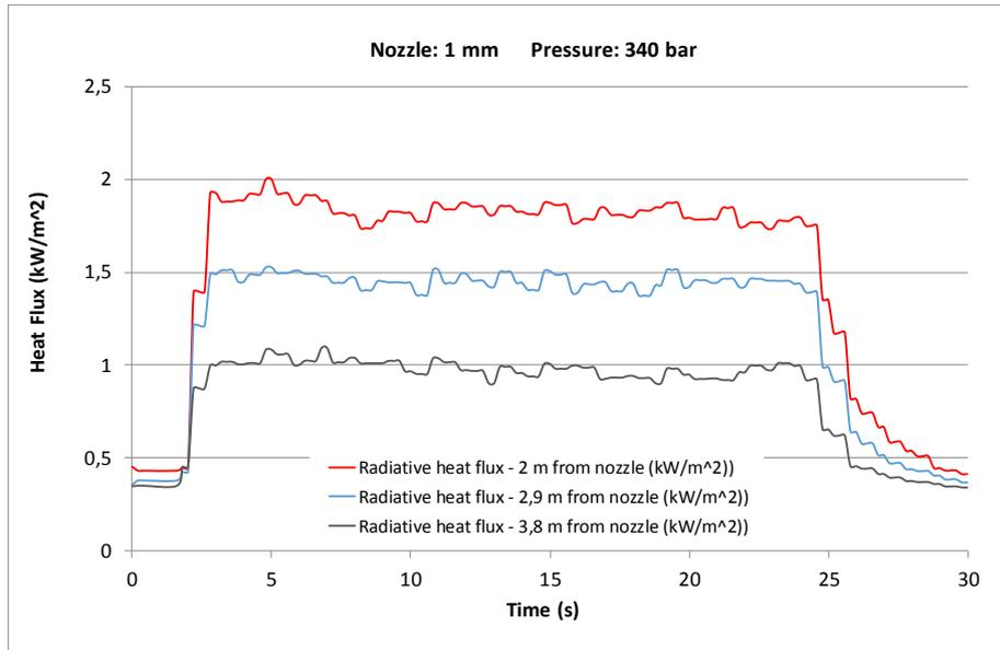
Figure 5: Heat Flux for 1 mm orifice at 340 bar.
