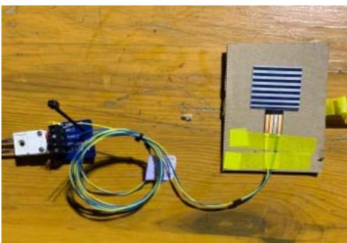
Figure 3: The Captec Radiant Flux sensor.
