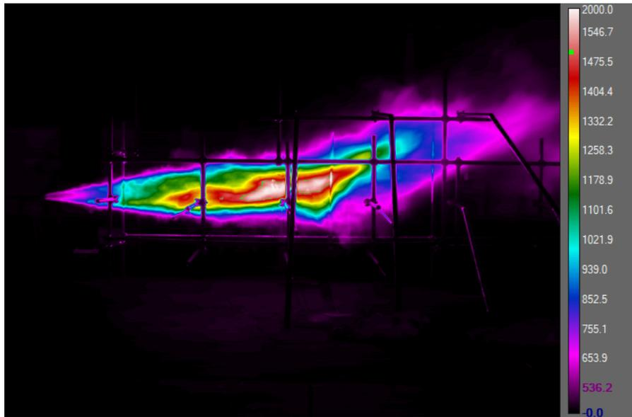
Figure 4: IR image of flame for test at 3 mm orifice and 325 bar (Temperature in K).
