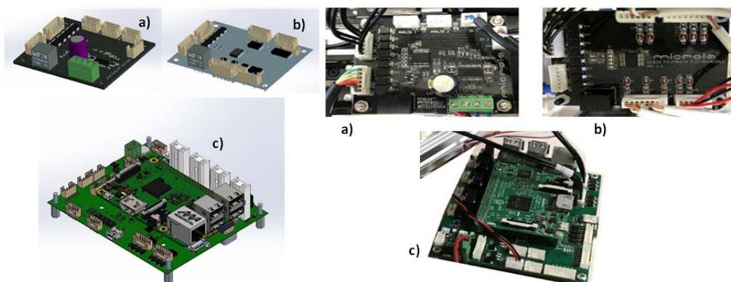
Figure 4: CAD renderings and realization of electronic boards: a) Moto-syringes board, b) valve board, c) motherboard.
